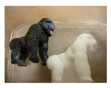
Figure 4: 2 Gorillas, on the left, plastic made black Gorilla. On the right, ultrasound friendly material.
