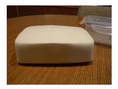
Figure 3: The ultrasound block with a plate underneath, covered with a skin like material
